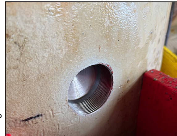
Wellhead Tapped - 2" Line Pipe Thread
