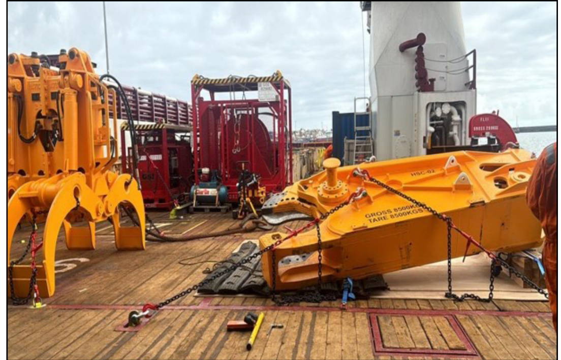
Claxton Pipe Grab and Cutting Shears on vessel deck
