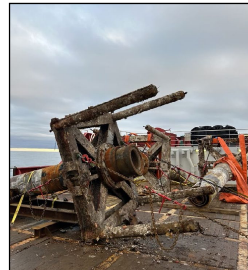
Recovered single & multi-string wellheads
