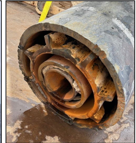
Cut four string casing with cement & centralisers
