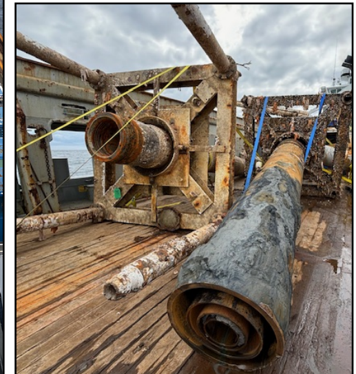
Recovered single & multi-string wellheads
